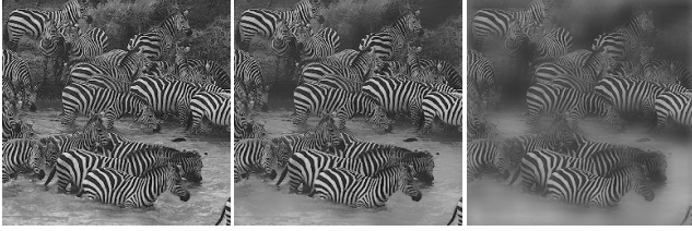
Figure 8. Effect of different range kernel variances for ArBs box filter: original, \sigma_r^2=0.02 , \sigma_r^2=0.2 at r = 10 .
